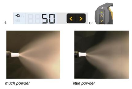
Adjust the powder output volume (e.g. according to the desired coating thickness)
