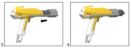
Insert the SuperCorona ring on the threaded sleeve (3) and connect it to the SuperCorona connection (4).
