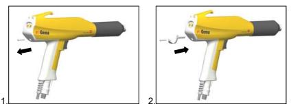
Fasten the SuperCorona connection with the existing screw on the rear side of the gun (1 and 2).
